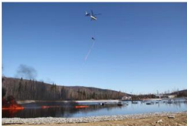
Figure 5. Heli-torch operation over basin during Test 5.
