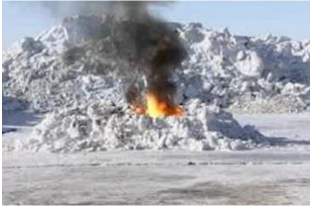
Burning oiled snow in volcano-shaped piles. Source: Alaska Clean Seas
