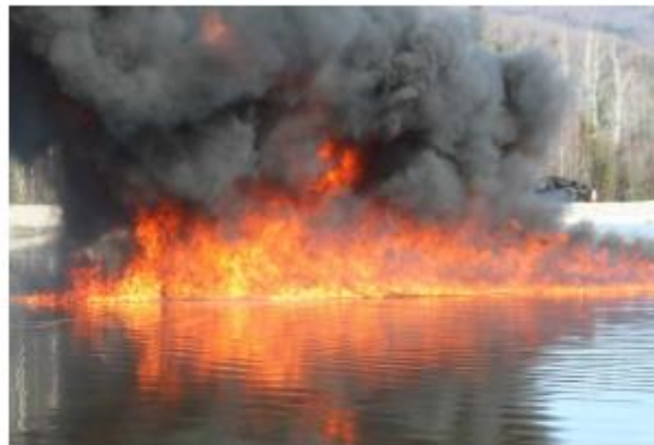
Figure 7. Successful burn of free-floating ANS slick herded with TS 6535 in Test 5.
